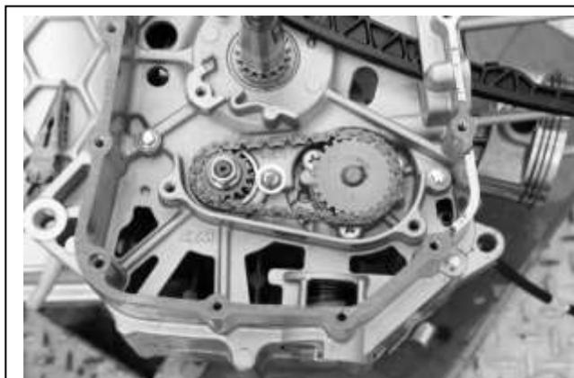
Install the oil separator (bolt x2).
