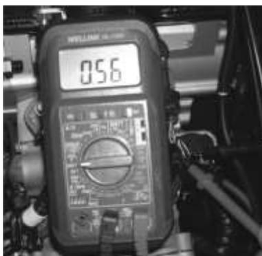
TPS output voltage – throttle fully closed
