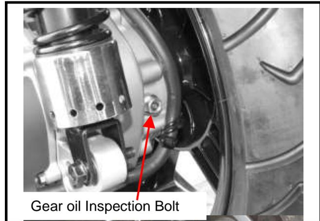
Gear lubrication oil quantity has to be measured with measurement device.
