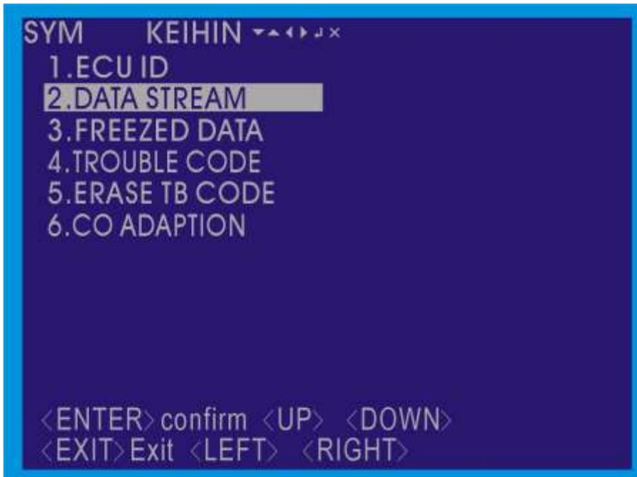
A total of 3 pages, are able to use "◀ left" and "right ▶" button, view injection system information. On the any screen, press the "EXIT" button, the function can return to the directory screen.
