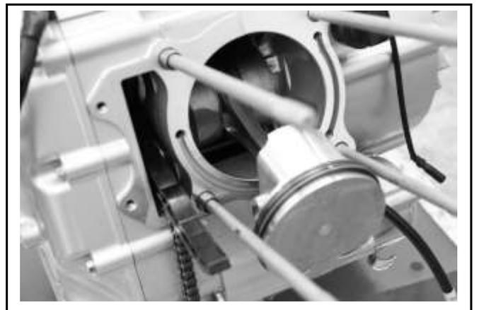
Install dowel pins and new cylinder gasket.
