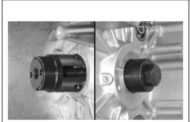
Fix the remover with the universal holder and press out the main bearing.
