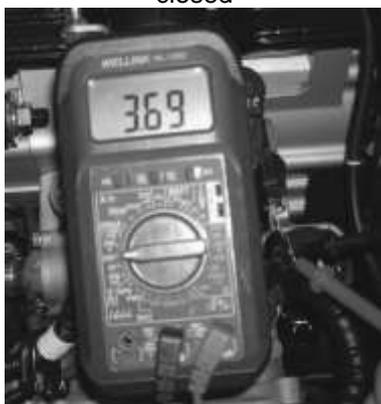
TPS output voltage – throttle fully opened
