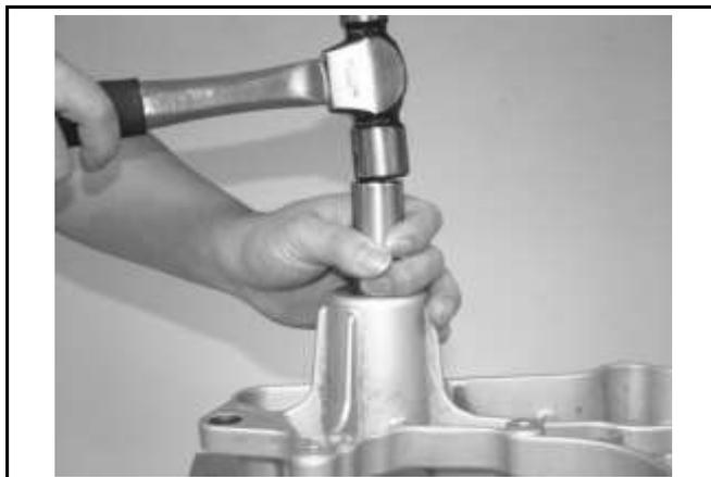
Install new rear fork bearing and bearing puller (6303) onto rear fork.
