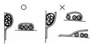
• Do not squeeze wires against the weld or its clamp.
