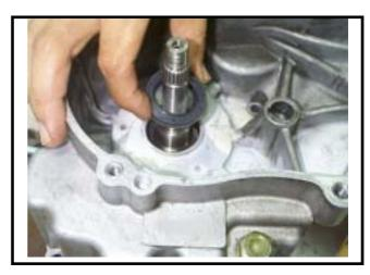
Press-fit the oil seal to specified position with the oil seal installer (25x37x6). **Special service tools: the oil seal installer (25x37x6)**
