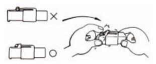
Check if the connector is covered by the twin connector boot completely and secured properly.
