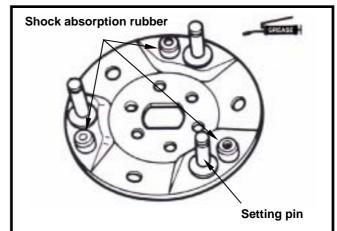
Apply with grease onto setting pins. But, the clutch block should not be greased. If so, replace it.
