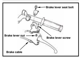
With a wrench to hold the handlebar bolt and then remove the nut.
