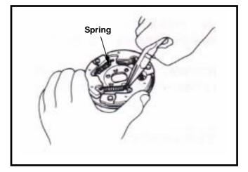
Install snap ring and mounting plate onto setting pin.
