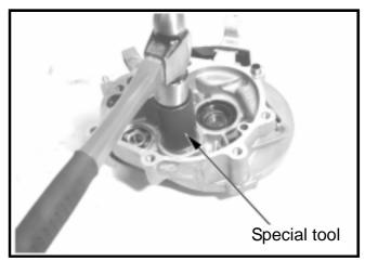
Press out the driving shaft from the
