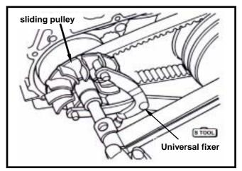
Hold driving pulley with universal fixture, and remove nut and clutch outer.
