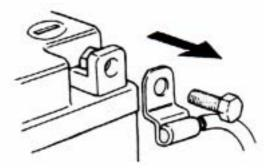
After service completed, make sure all connection points is secured. Battery positive (+) cable should be connected firstly. And the two posts of battery have to be greased after connected the cables.
