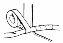
• Secure the rubber boot firmly as applying it on wire harness.
