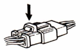
• Do not pull the wires as removing a connector or wires. Hold the connector body.
