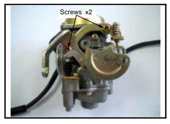
Remove the accelerate pump drive arm from the carburetor.
