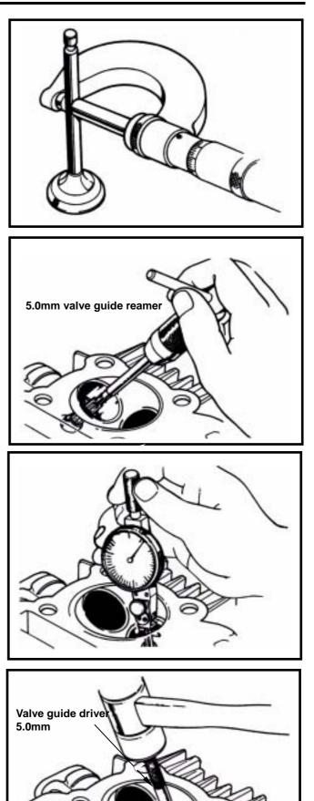
Hold the cylinder head, and then press out old valve guide from combustion chamber side. **Tool: Valve guide driver 5 mm**
