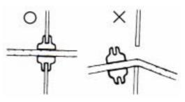
Never use wires or harnesses which insulation has been broken. Wrap electrical tape around the damaged parts or replace them.
