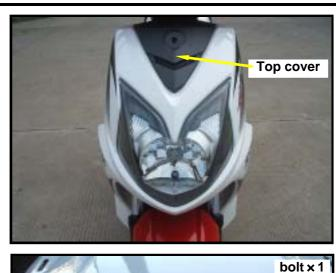
Remove the 1 mounting bolt of front cover from the frame.
