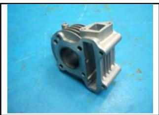
Remove cam chain plate. Remove cylinder.
