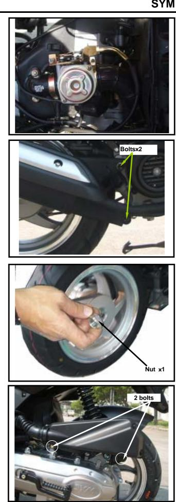
Remove the rear brake cable nut. Remove the rear brake cable. Remove the rear shock absorber lower bolt.
