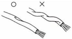
• Wire harnesses routed along the handlebar should not be pulled too tight or have excessive slack, be rubbed against or interfere with adjacent or surrounding parts in all steering positions.
