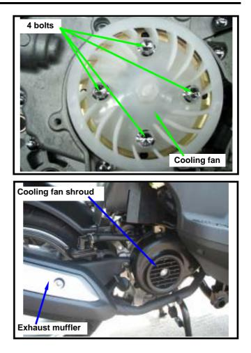
Install the cooling fan shroud. (4 bolts) Install the exhaust muffler. (2 bolts, 2 nuts) Add some engine oil according the specified quantity.
